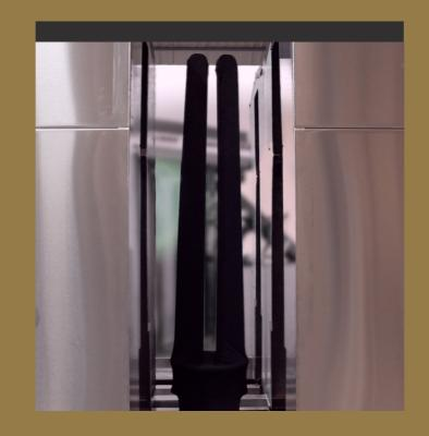
Washing/drying is in a closed booth system with 100% recirculation of water and heat, creating no waste or effluent.
