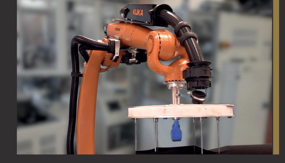
From knitting, the legs and bands are brought together through an automated collection point and then moved by robot to the sewing station.
